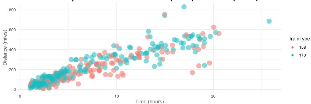
The data in Figure 10 can be split out by train class and by number of units, as shown in Figure 11. Approximately 200 trips for both Class 158 and 170 trains were recorded, with only 26 and 7 running in multiple trips, respectively.
