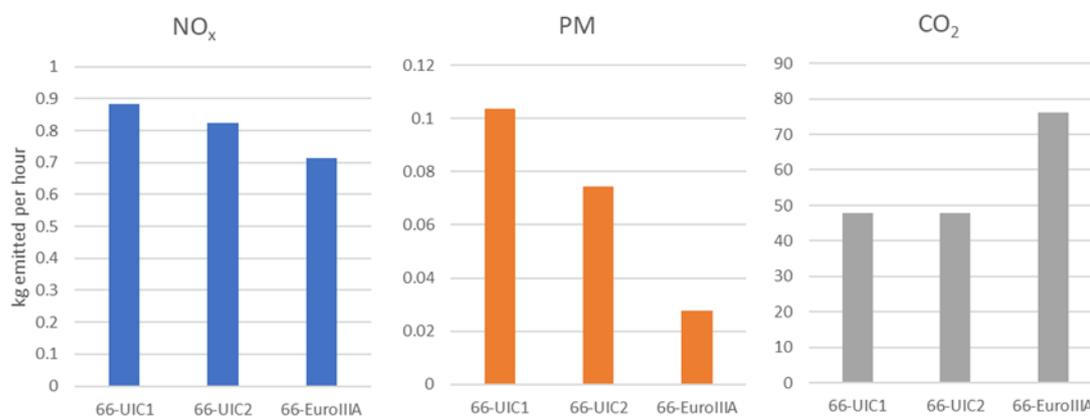
While a Class 66-UIC1 locomotive is idling, it emits 0.88 kg NO<sub>x</sub>, 0.104 kg PM and 47.8 kg CO<sub>2</sub> per hour.
