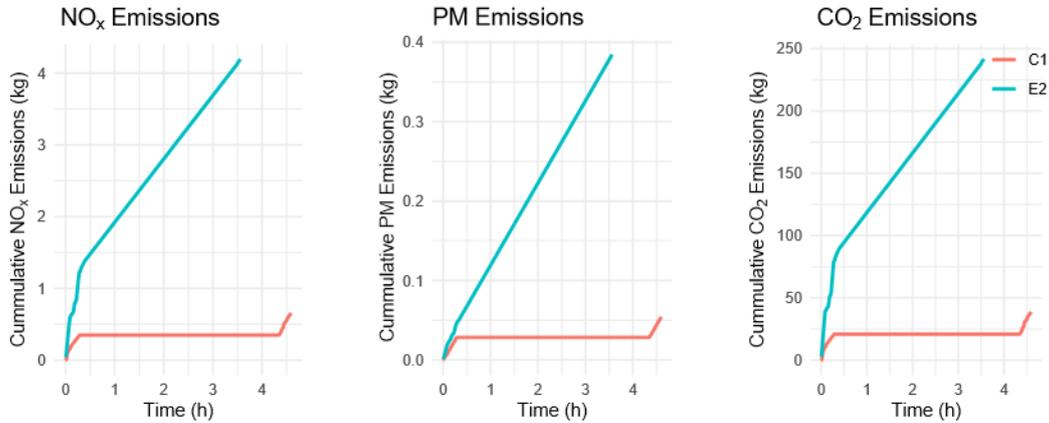
While the engine is left on, the emissions of all three pollutants continues to increase linearly, whereas the emissions flatline if the engine is switched off. As discussed in Section 4.1.5, PM emissions increase at the steepest proportionate rate while idling compared to NO<sub>x</sub> and CO<sub>2</sub>.
