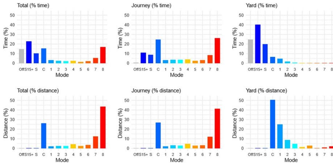
The results are as expected. In the Journey drive cycle, most of the time spent and distance travelled is in Notch 8 or coasting. In the Yard drive cycle, most of the time is spent in the Off, Stationary, or Stationary >15mins modes, and the limited distance covered is in lower notches. Unsurprisingly, no distance is covered when the mode is Off or Stationary.
