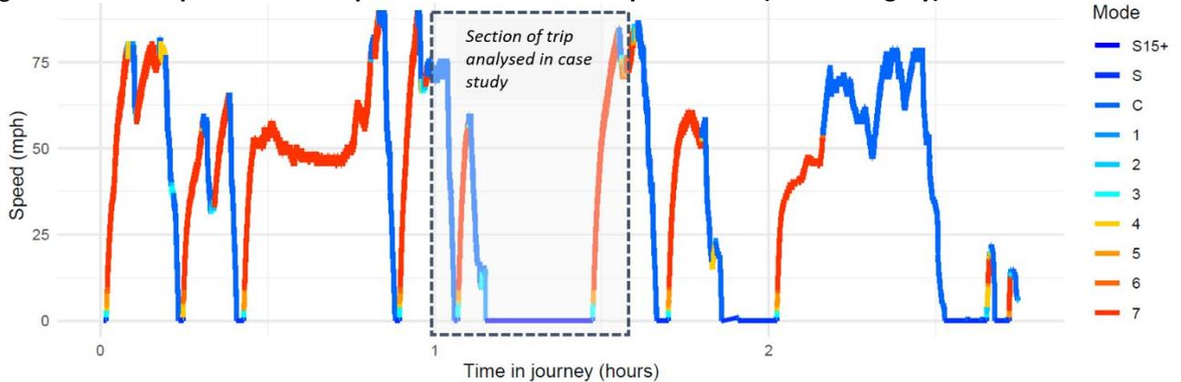
Figure 27 shows the highlighted section of the trip from Figure 26 in more detail. Between 1h00 and 1h30 into the trip the train stops at a station and idles for more than 15 minutes (Figure 27a). Table 12 presents an overview of the emissions generated over the entire 100-mile trip and during the period spent in continuous idle for over 15 minutes. For every 15 minutes spent in idle, approximately 60 g of NO<sub>x</sub>, 20 g of PM and 27 kg of CO<sub>2</sub> are generated.
