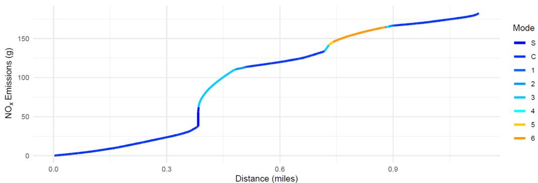
The NO<sub>x</sub> emissions generated in Examples 2 and 3 (the delayed approaches) were approximately three and five times greater than Example 1 (the smooth approach), respectively.
