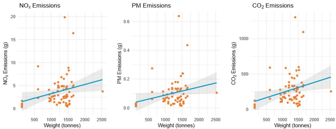
Most of the freight data have similar weights, clustered around 1000-1500 tonnes. However, the few examples with more extreme weights show that there is a positive trend: emissions from acceleration increase with train loading. More examples with a wider range of weights would help to clarify the exact nature of this relationship.
