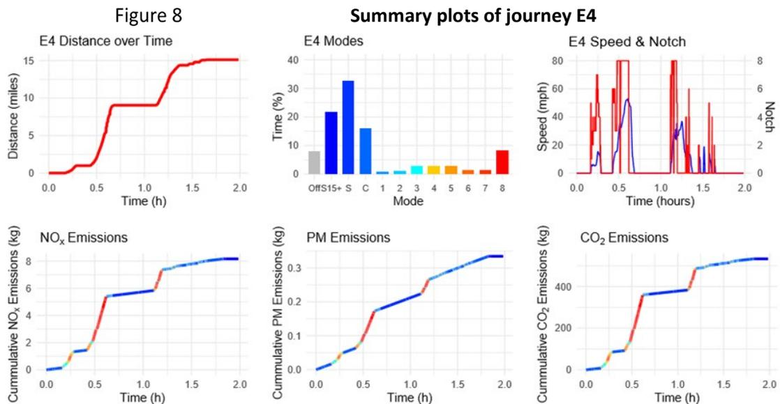
All emissions of this journey are significantly affected by the stationary period, but emissions of the three pollutants are not equally affected. PM continues to be emitted at a very high rate while the train is idling, while NO<sub>x</sub> and CO<sub>2</sub> continue to be emitted but at a lower rate. This is due to the large difference in idling and powered emission factors.
