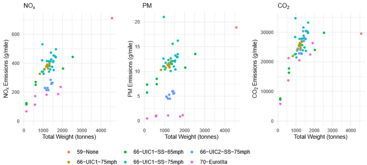
From the data shown in Figure 46, it appears that within each class there is an approximate linear relationship between emissions in grams per mile and weight. Importantly, this relationship shows that doubling the weight of the train does not double its emissions (gradient is less than 1). The outlier discussed in Section 4.1.5, journey E4 at 961 tonnes, is a very short and slow journey with a large amount of intermediate stationary time.
