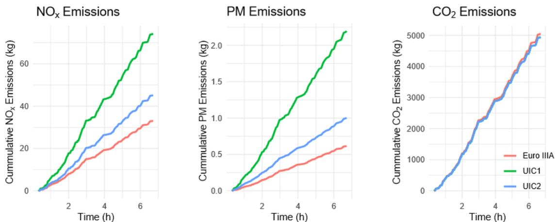
The NO<sub>x</sub> and PM emissions reflect the evolution of the three emission standards, with the largest difference for PM between UIC1 and UIC2<sup>18</sup>. The UIC1 and UIC2 CO<sub>2</sub> emission factors are the same so these lines cannot be differentiated in Figure 49, while the Euro IIIA CO<sub>2</sub> emission factor is slightly higher so trip CO<sub>2</sub> emissions are slightly higher.
