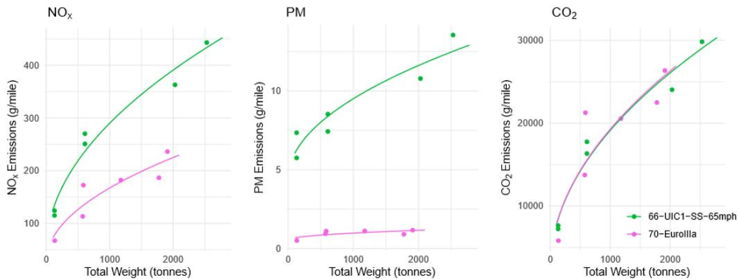
Figure 48 shows the emissions for the same two classes of locomotive plotted as g/t-m against weight. A  $1/\sqrt{x}$  model was fit to each set of points, since there will be the same relationship modelled in Figure 47<sup>17</sup>.
