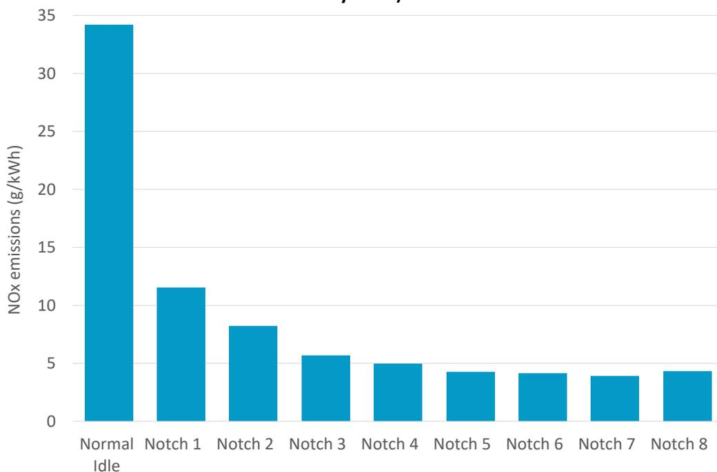
Figure 2 **NO<sub>x</sub> emissions in kg/hour for the EMD 710 V12 Euro IIIA specification engine**
