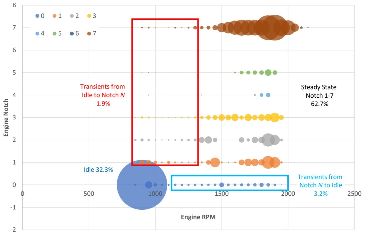
Drive cycle weightings for all rolling stock types and engine/transmission variants in scope for the project were derived by blending the audio and OTMR data together and are provided in the associated Spreadsheet 1.
