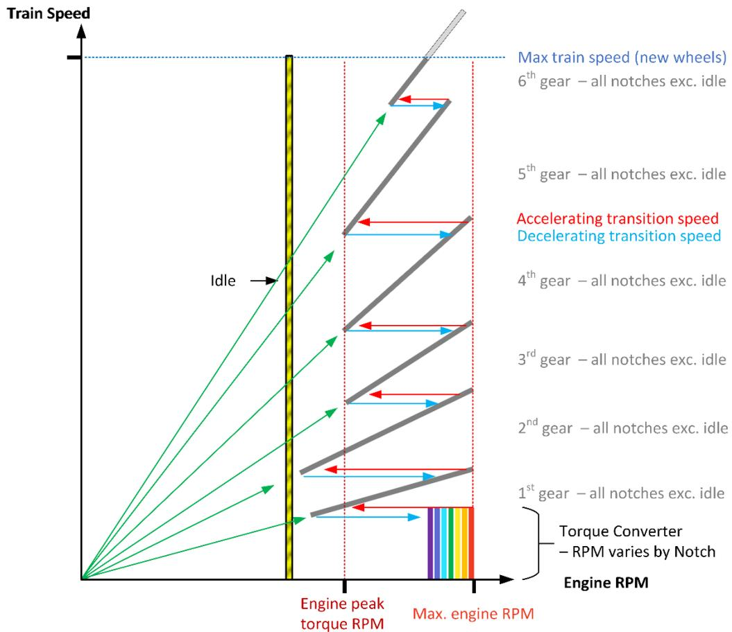
In the higher gears the engine operates in the range between engine peak torque and maximum engine rpm. In first and second gears (at the lower train speeds for those gears) the engine operates below the peak torque point under non transient condition, an operating condition that does not occur with hydraulic transmissions. This situation is illustrated in Figure 19 by the two black ellipses.
