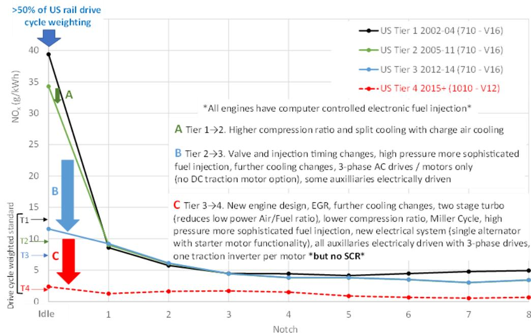
To measure a reduction in emissions as part of total use or specific situations, it is necessary to aggregate emissions from different mode test points and apply a weighting. The Testing Protocol requires flexibility in weightings and so needs a time-based approach, which focuses attention on the effectiveness of solutions in real circumstances.
