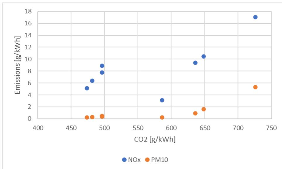
**Figure 4:** NOx and PM emissions vs CO<sub>2</sub> emissions
