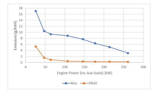
Figure 3: NOx and PM emissions vs engine power
