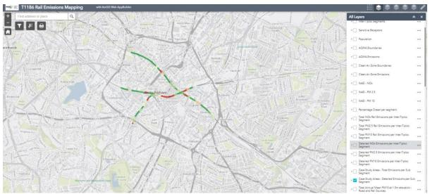
Figure 8: Emissions predictions in the central Birmingham area using notch-based emission factors
