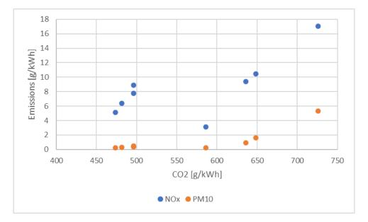
Figure 4: NOx and PM emissions vs CO2 emissions
